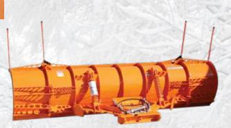
Bonnell Bat Wing snow plow extensions provide that extra width for fast and efficient snow removal, while retaining the mobility necessary to travel from site to site. One pin operation provides simplicity for the operator to transform the plow into a width of 14' to 18' depending on the base length of the plow. Versatility is the name of the game, and Bonnell Industries can help you get the job done.
